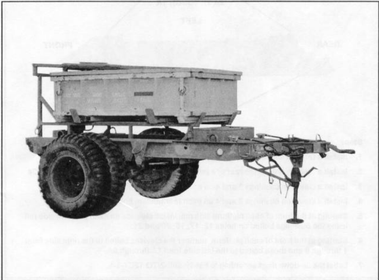
Figure 5-1. Unrigged MICLIC on 2 1/2-ton trailer
